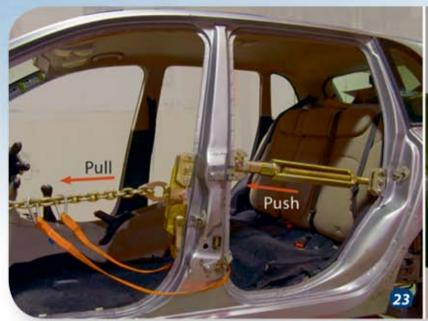
In line straightening of the strong-structured B pillar often requires a hydraulic pull together with a simultaneous mechanical push.
