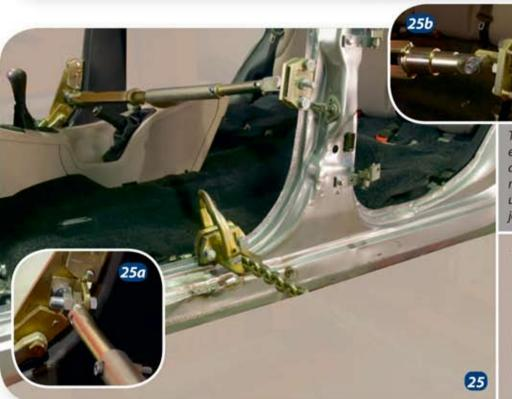
The B pillar straightens out more easily, if a support is placed at the damaged point. The support equipment shown in the picture can also be used in other kinds of straightening jobs.
